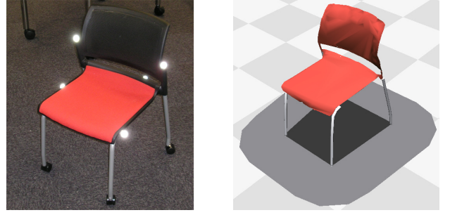
Fig. 3. (a) Chair used in our experiments with retro-reflective markers illuminated. (b) 3D model of the chair. The dark ground regions represent the planar obstacle and the \mathcal{C} -space obstacle. The robot may walk on the grey region, but its torso COM must not enter it.
