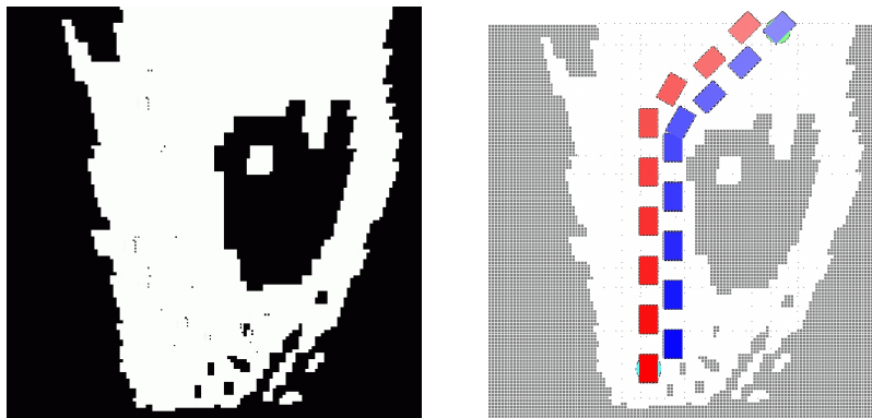
Fig. 13. Online footstep planning: ( top row: H7 humanoid and candidate walking surface area extracted from 3D stereo depth map; bottom row: distortion-corrected obstacle map after thresholding, and calculated optimal footstep sequence to target.
