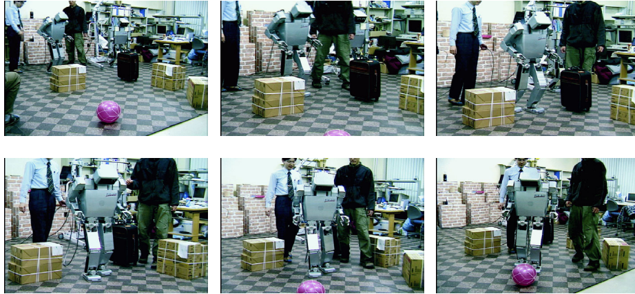
Fig. 14. Snapshots of the humanoid H7 calculating and executing online the footstep sequence from Figure 13
