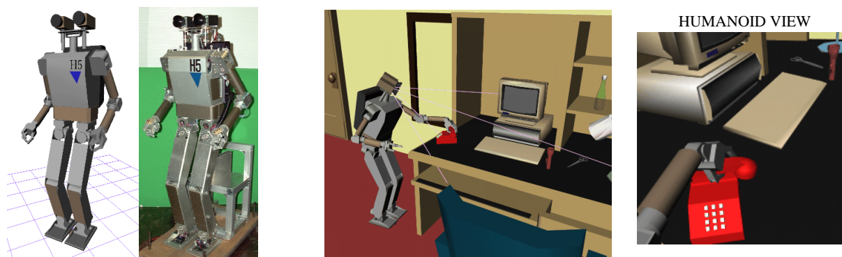
Fig. 1. The virtual and real dynamic humanoid 'H5' (left), and answering the phone in a simulated world (right).
