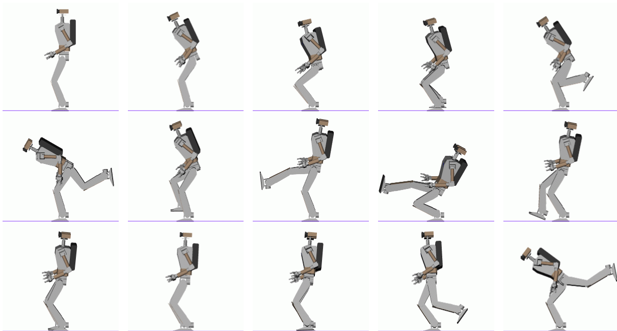
Fig. 6. Dual-leg and single-leg stable postures for the H5 humanoid robot (left view).
