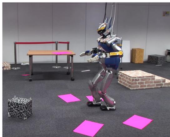
Fig. 1. The HRP-2 humanoid navigating autonomously through a set of obstacles during vision-guided walking.
